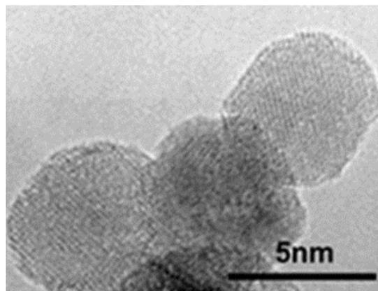
**Figure 1:** High Resolution TEM (HRTEM) image of primary particles of detonation nanodiamond (DND).
