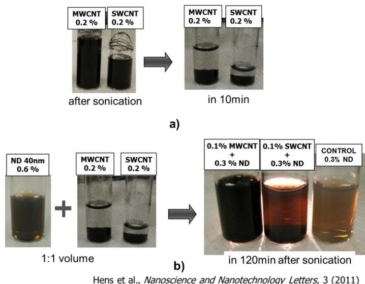
**Figure 10:** Photographs showing the colloidal stability of suspensions for SWCNT and MWCNT in water without (a) and with DNDs (b).
