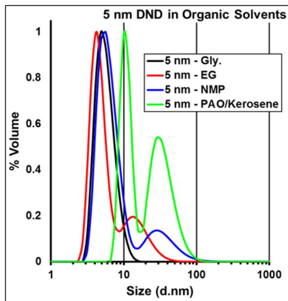
**Figure 7:** Volumetric DLS spectra of 5 nm particles in a variety of organic solvents.
