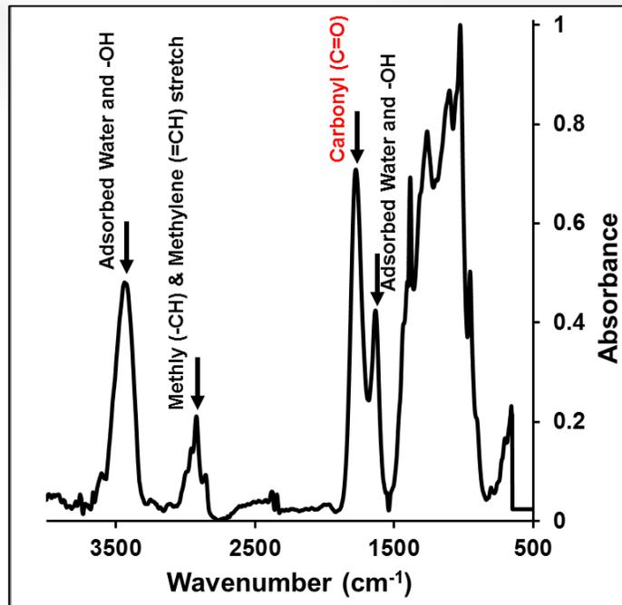
**Figure 3:** FTIR of carboxylated 5 nm material.
