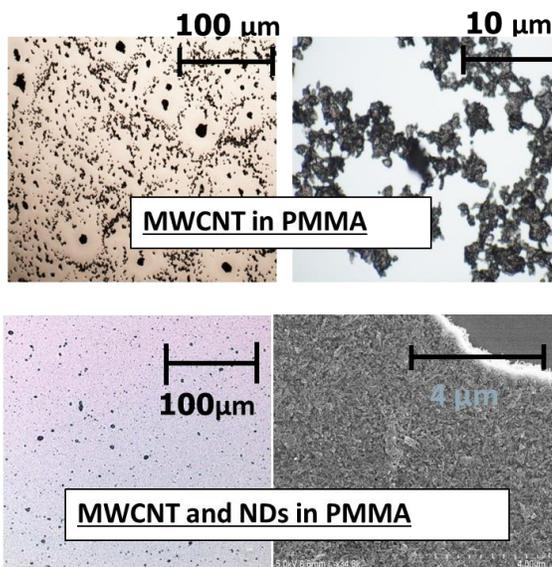
**Figure 11 (right):** Excellent uniformity of CNT distribution within a polymer film can be obtained with assistance of NDs.
