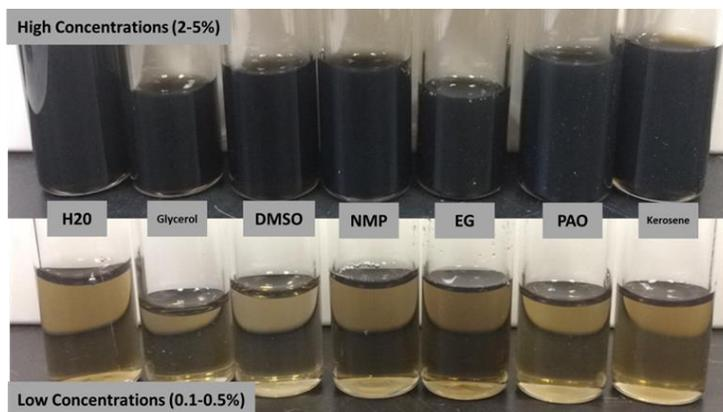
**Figure 8:** Dispersions of 5 nm particles of DND in a variety of organic solvents at high concentrations (2-5% w/v) and low concentrations (0.1-0.5% w/v). High colloidal stability in a variety of solvents provides functionality in a large number of applications.
