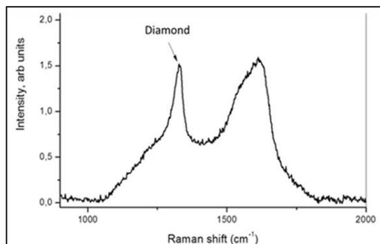
**Figure 2:** Raman spectra of 5 nm DND showing characteristic DND Raman peak at 1327 cm<sup>-1</sup>. Courtesy, I. Vlasov.
