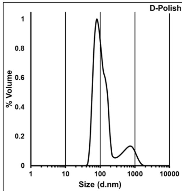
**Figure 12:** Volumetric DLS size distributions of D-Polish suspension diluted in deionized water.
